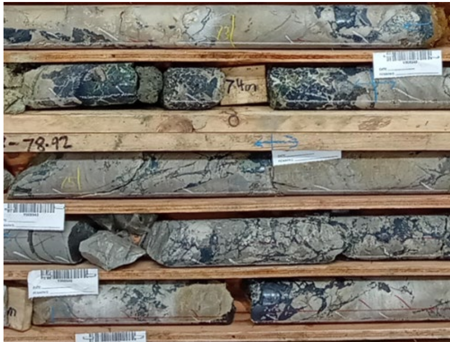
Figure 4: Dense semi-massive and breccia visual chalcocite (dark grey mineral) from PFS-002 (72.7-76.5m downhole). This interval assayed at an average grade of 8.3% Cu, 31g/t Ag.
