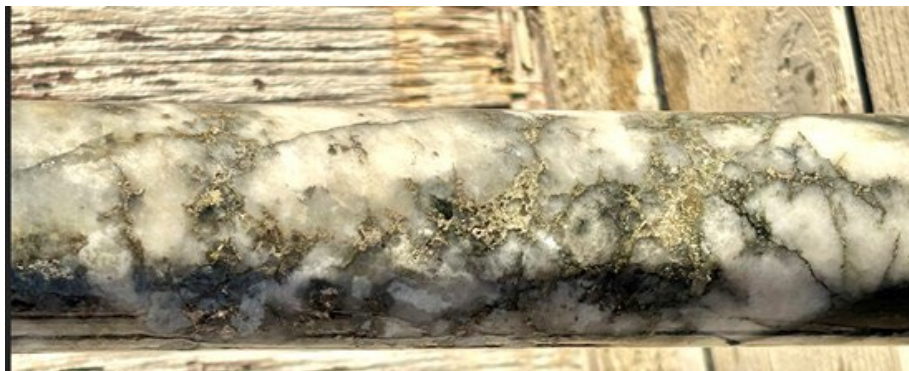
Image 1: Net Texture Sulphides in Quartz Veining from 25UND002.
